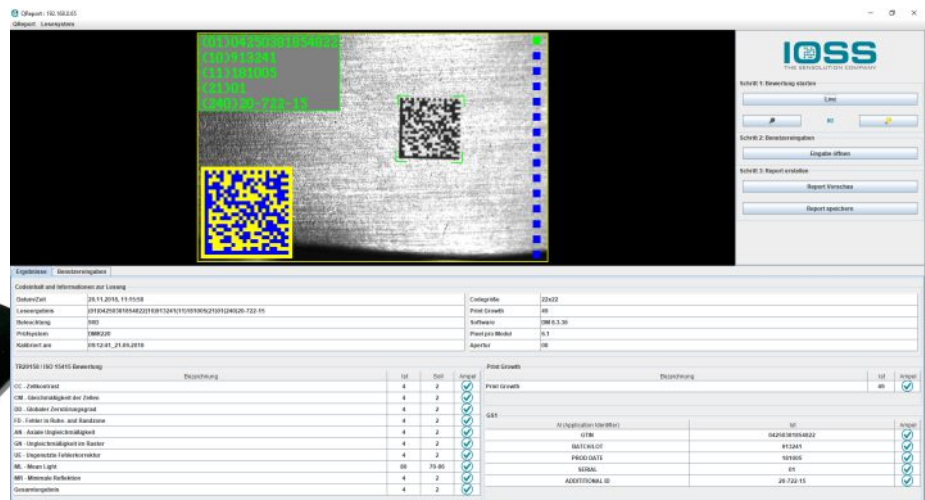
Q-Report: Documentation software as proof of the quality and readability of the data matrix code
